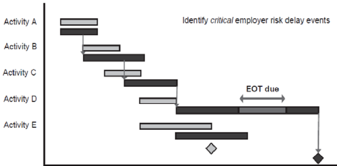
Figure 3.16 Comparative as planned and as built programmes – delay identified.
